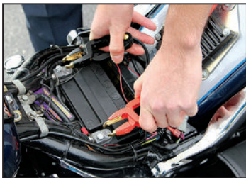
Detach Clamps From Battery
