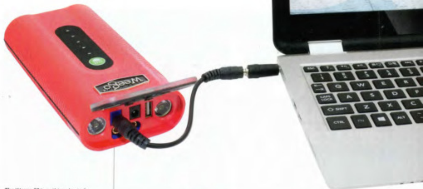
› Above: The optional Laptop Charger Connector accessory allows charging most laptop computers directly from the Weego 44's 19V connection.
